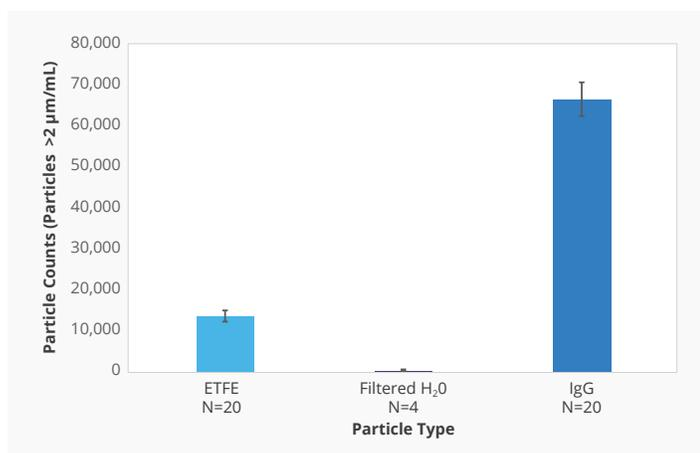
**FIGURE 1:** Low volume analysis of polydisperse samples in BMI. 25  $\mu\text{L}$  samples of ETFE and IgG were measured with 20 replicates each. CVs for ETFE and IgG samples were 9.7% and 6.2%, respectively.
