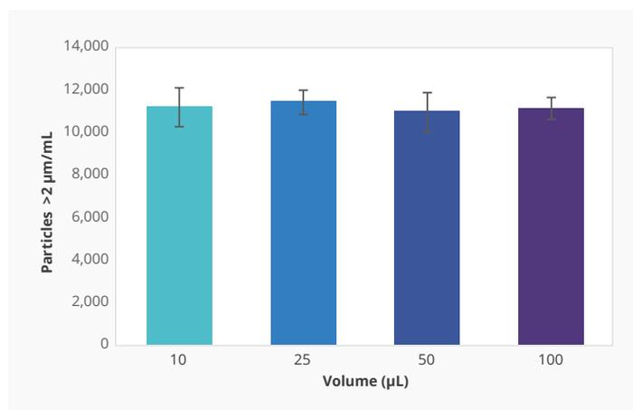
**FIGURE 2:** Impact of volume on polydisperse samples in BMI. Varying volumes of ETFE samples were measured. Particle counts were all within 4% of each other, demonstrating sample volume did not impact measurement precision.
